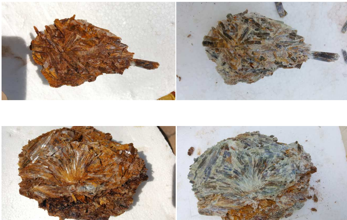
Specimens before and after cleaning: Upper cleaned with Iron Out+sodium citrate and lower cleaned with oxalic acid in a slow cooker (keep warm setting). Pictures taken with Samsung S6. pounder
